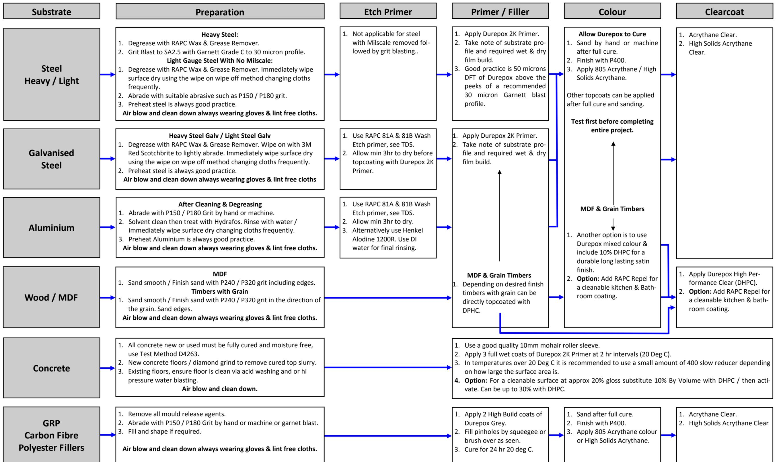
Durepox 2K primer is a very unique 2 pack epoxy Urethane that can be applied by brush, roller, airless, air assisted airless, electrostatic and conventional gravity or pressure pot spray. Durepox has many applications from hi build primers to being used as coloured topcoats in conjunction with Durepox High Performance Clear (DHPC). Other 2K topcoats can be applied over Durepox after full cure and sanding, test an area first before completing entire project.
